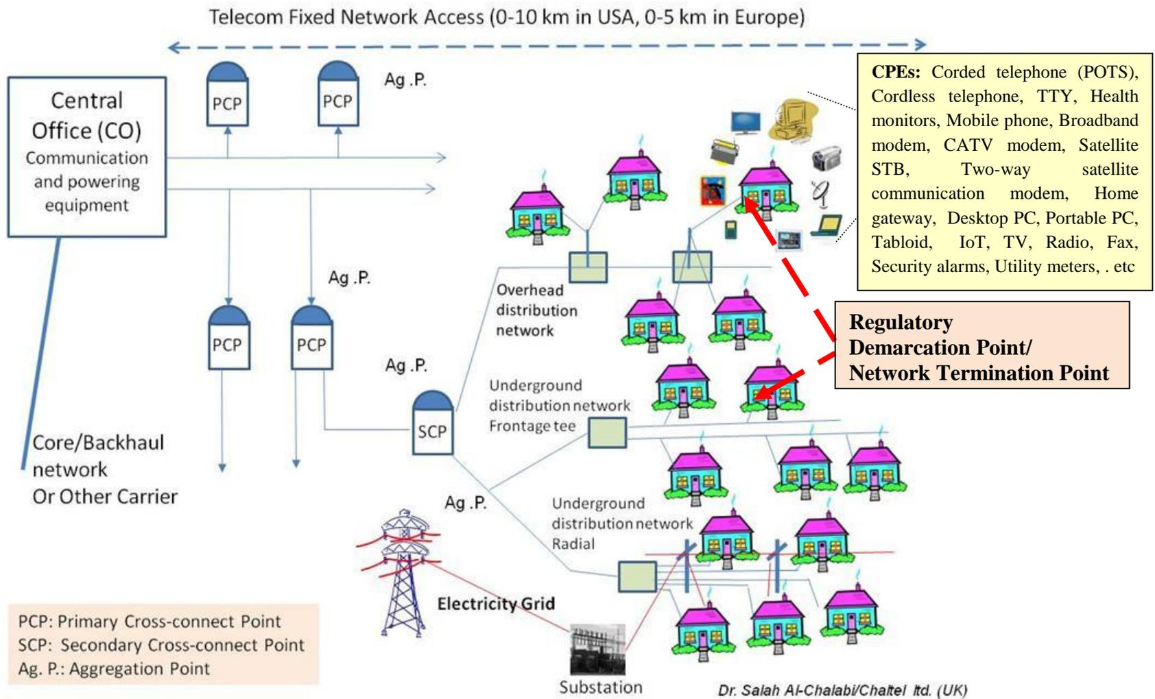
Figure 3: Telecom Public Fixed Access Network and Local Electricity Grid
