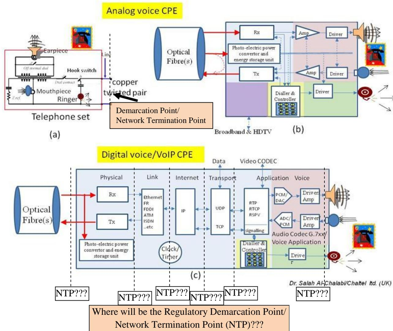
Figure 5: Essential components of telephone CPE (a) copper-based analog telephone with centralized powering (b) fiber-based analog telephone with centralized optical powering (c) fiber-based digital VoIP telephone with centralized optical powering
