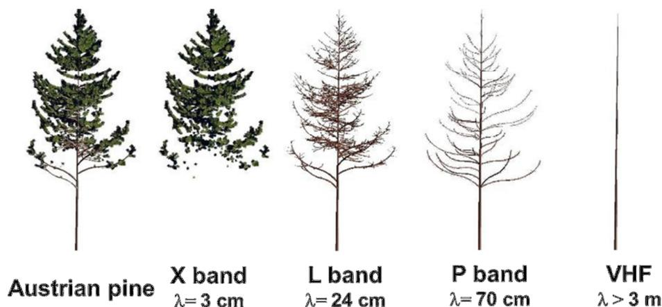
**Figure 6 – Radar returns from vegetation at various wavelengths**
