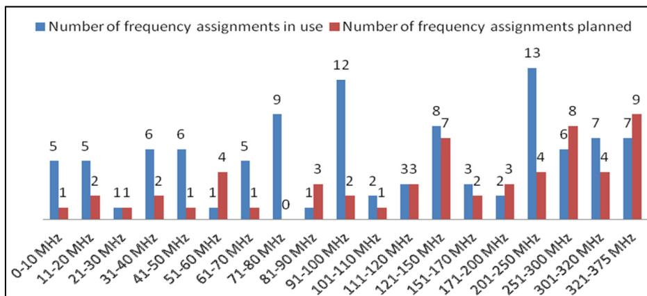
**Figure 11 – Bandwidth utilisation for the 8 025 – 8 400 MHz spectrum by science satellites (SFCG).**
