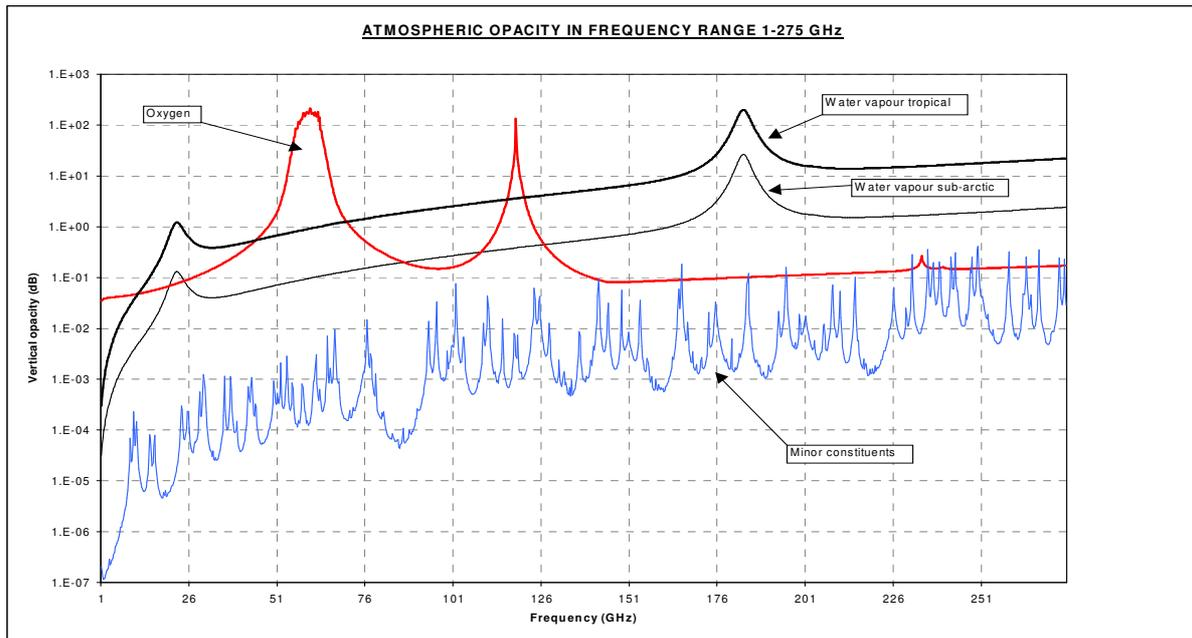
**Figure 5 – Atmospheric opacity 1 – 275 GHz**
