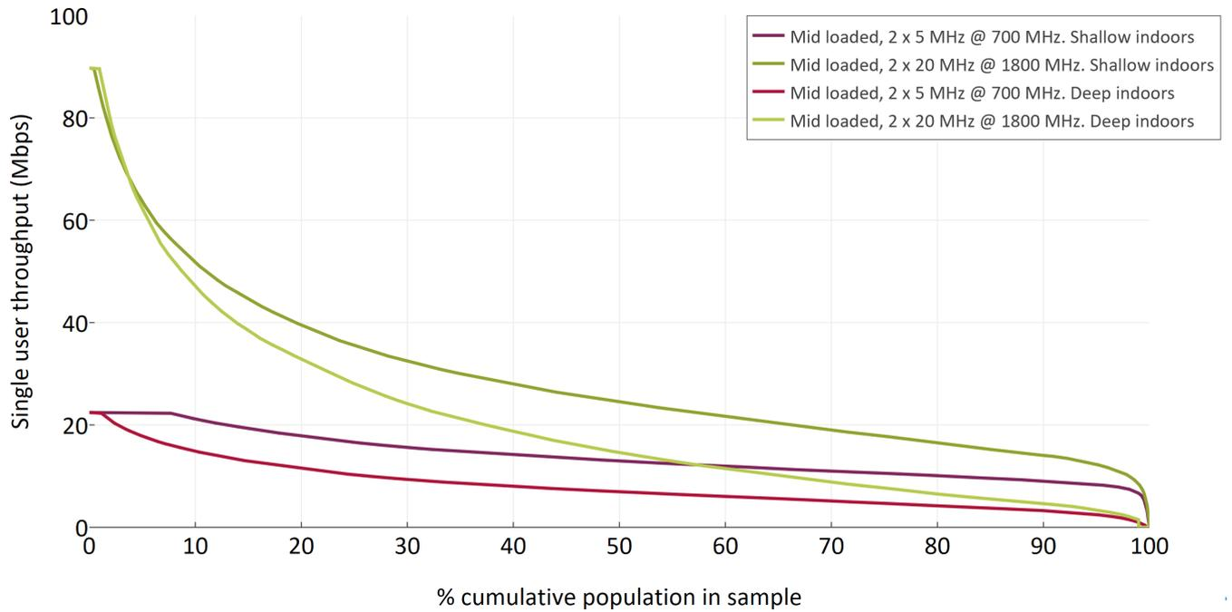
Figure A10.11: SUT distribution curves, shallow and deep indoor locations in mid densely populated areas (2 x 5 MHz of 700 MHz and 2 x 20 MHz of 1800 MHz)
