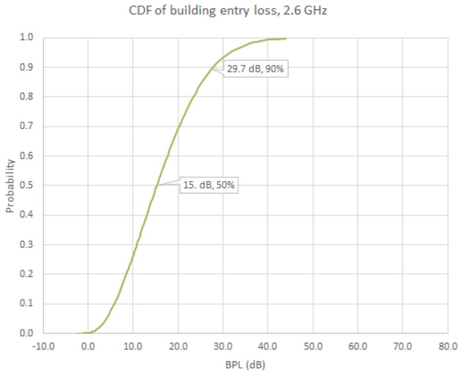
Figure A8.2: Building entry losses from ITU-R P.2109
