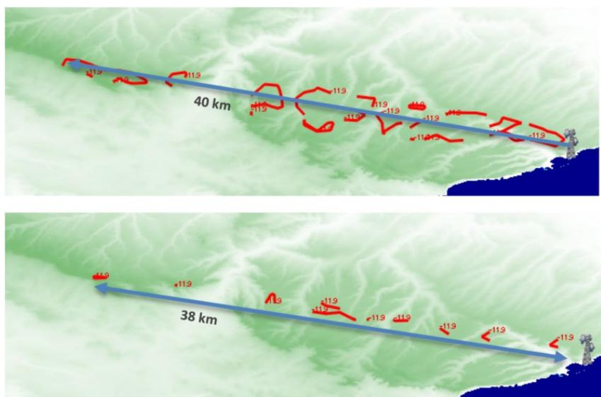
Figure A15.10: FL 2 worst-case (top) and realistic-case (bottom) interference contour for AAS
