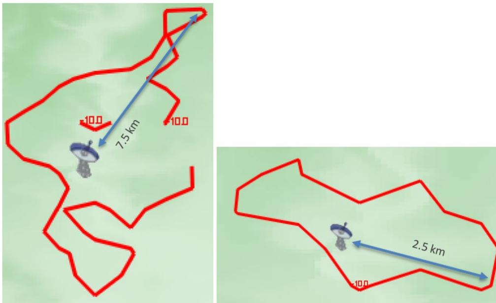
Figure A15.7: SES 3 worst case (left) and realistic case (right) interference contour for AAS
