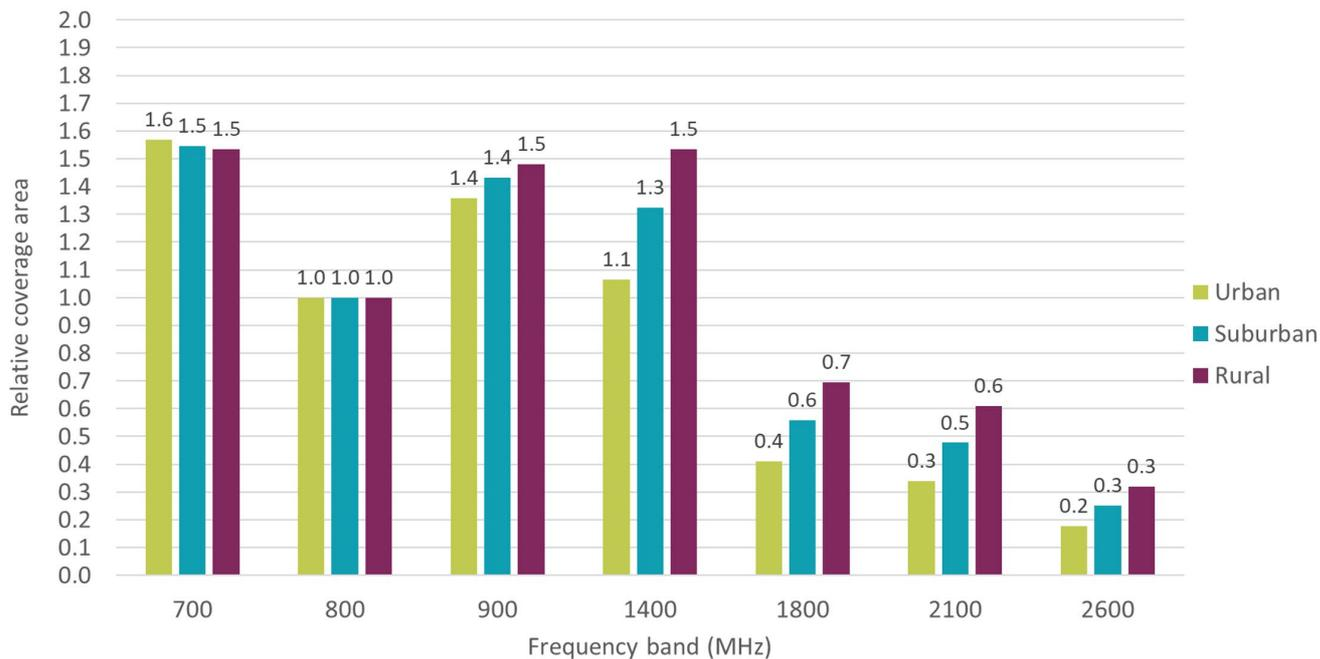
**Figure A8.4: Relative potential coverage estimated for the 90th percentile of building entry loss in deep indoor locations, normalized to 800 MHz coverage**
