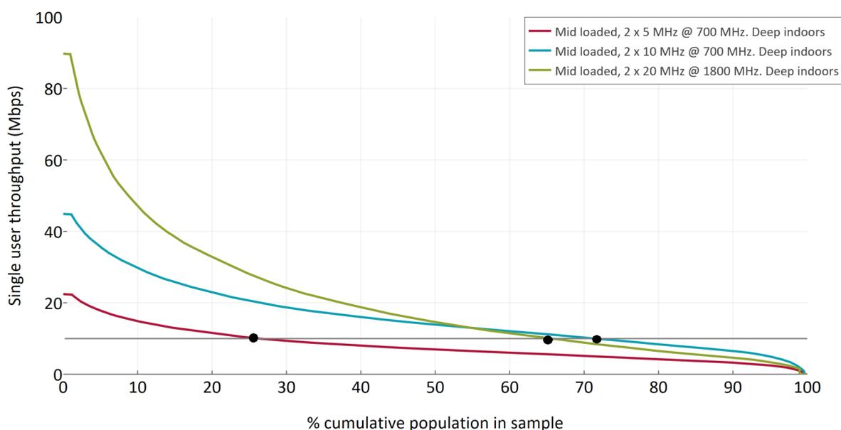
**Figure A10.13: SUT distribution curves, deep indoor locations in mid densely populated areas (2 x 5 MHz of 700 MHz, 2 x 10 MHz of 700 MHz and 2 x 20 MHz of 1800 MHz)**
