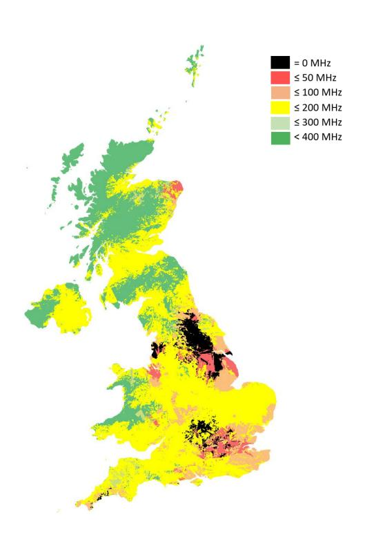
Figure 2: 2019 approach, total bandwidth available to a Medium Power user (3.8-4.2 GHz)
