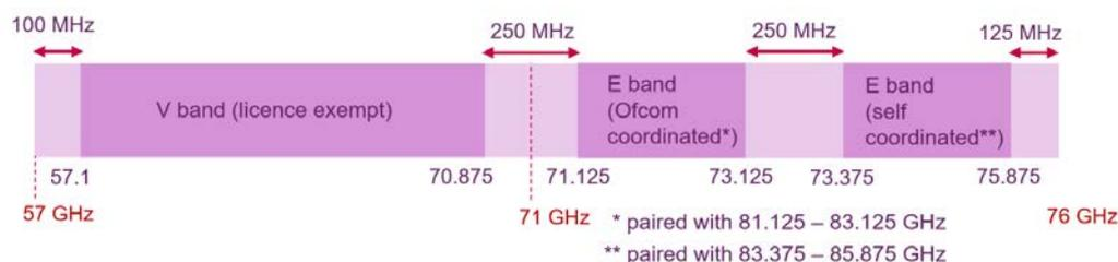
Figure 3: Frequency separation below 71 GHz
