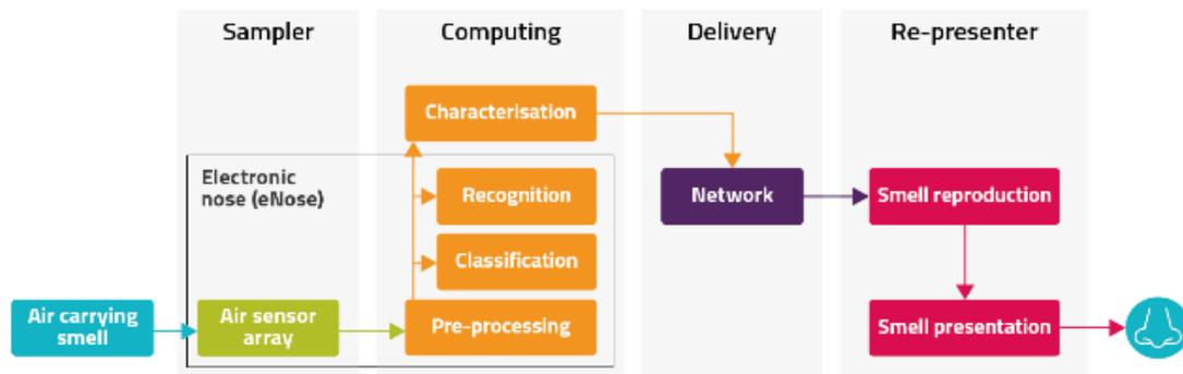
Recently, researchers at Intel and Cornell University have successfully used neuromorphic chips to develop an electronic nose that can learn the scent of a chemical after just one exposure to it and then identify that scent even when it is masked by others [Moore2020].
