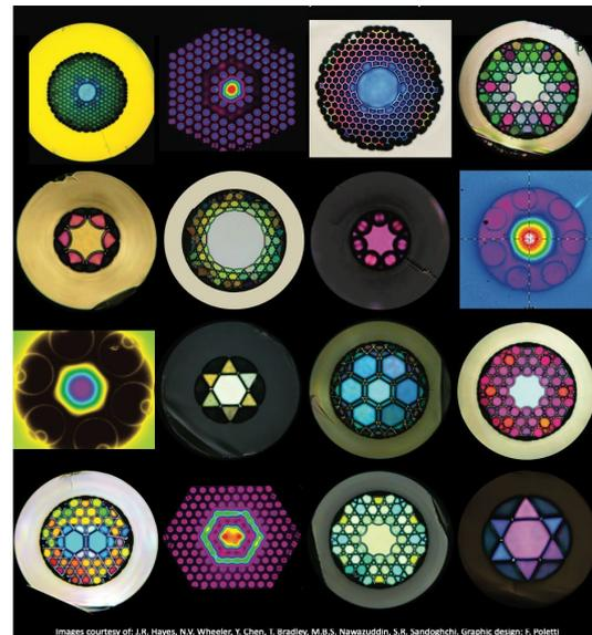
The resulting guided mode has only a tiny fraction of a percentage of its power in the glass (in the membranes). It is this last aspect that is important in most applications. Advantages are:
