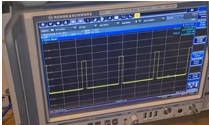
**Figure A1.2: Simplified waveform giving similar results in three TV receivers**
