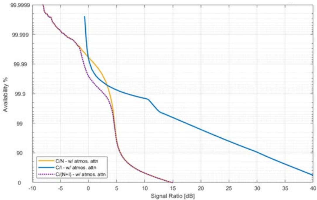
**Figure 3. Downlink Case 1: C/N, C/I & C/(N+I) of Starlink System**
