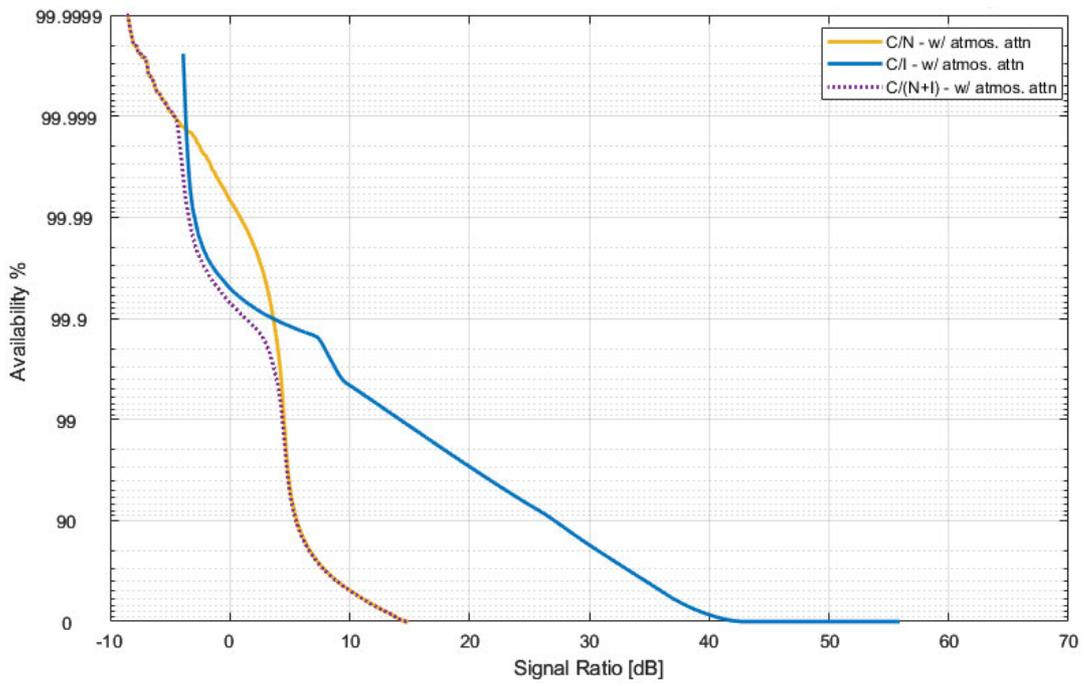
Figure 4. Downlink Case 2 C/N, C/I & C/(N+I) of Starlink System
