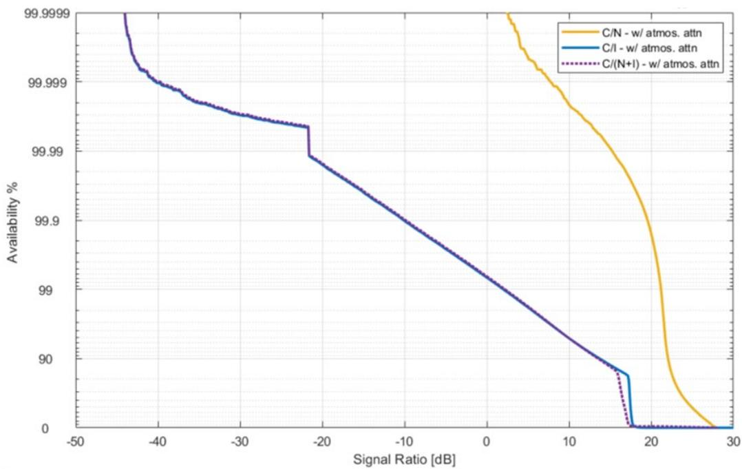
**Figure 1. Uplink Case 1: C/N, C/I & C/(N+I) of Starlink System**
