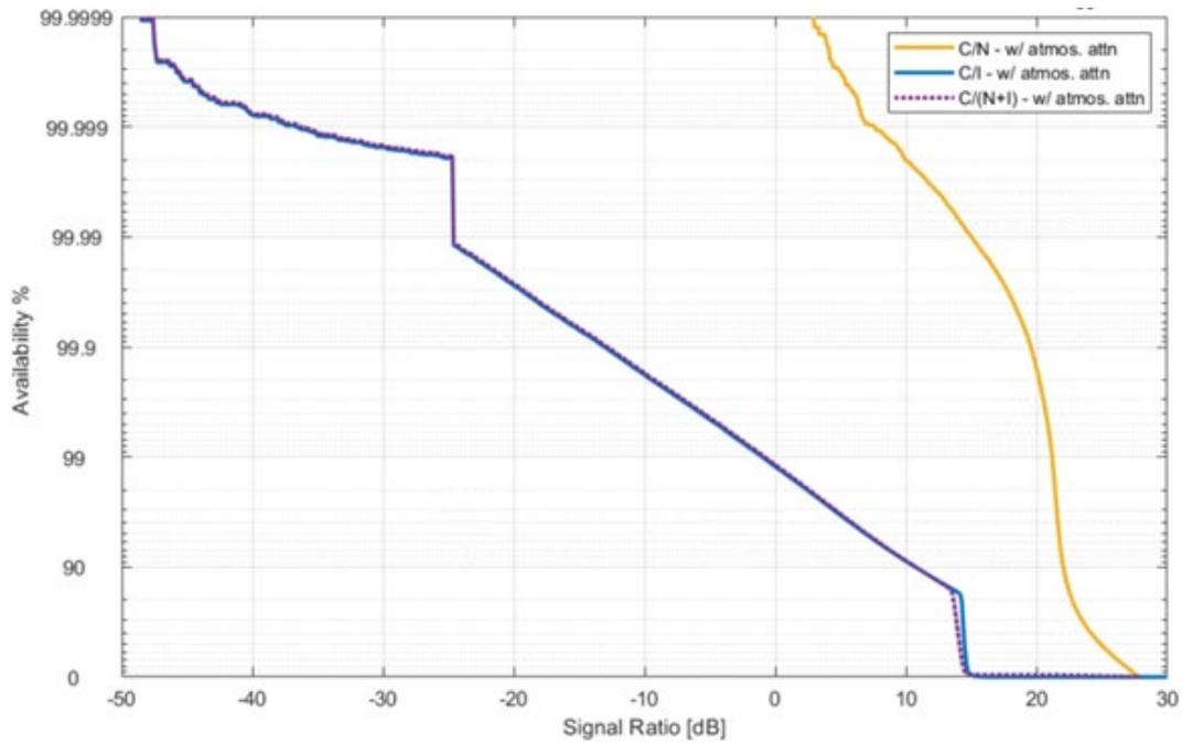
Figure 2. Uplink Case 2: C/N, C/I & C/(N+I) of Starlink System
