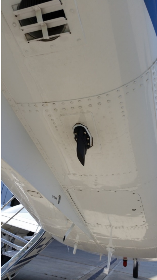
Figure 6: We mounted the antenna towards the back of the aircraft. The antenna is approximately omni-directional and we discuss its gain pattern in more detail in Annex 3. Note the “fin” shielding the antenna on the left side which is almost but not exactly parallel to the antenna and also the forward slope of the antenna mounting; we made sure to take these into account in our subsequent analysis. This antenna is connected to a Rohde & Schwarz FSW spectrum analyser inside the aircraft taking one RMS power scan every 10 seconds. We also used a mini-circuits ZFBP-2400 (2300 – 2500 MHz) filter to reduce the risk of overload from aeronautical transmitters on the aircraft itself.
