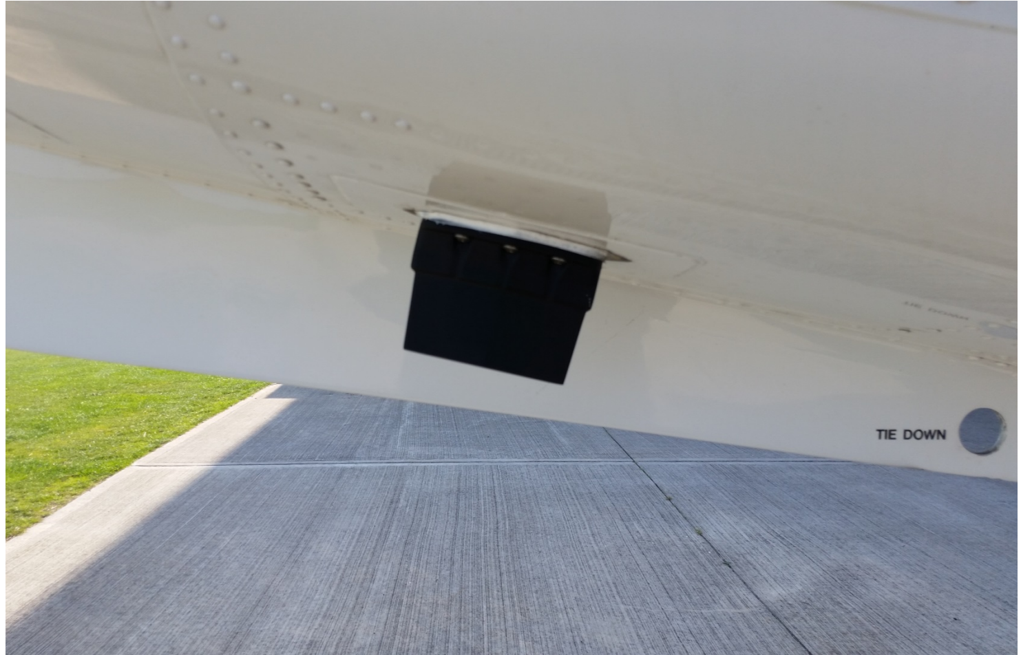
Figure 6: We mounted the antenna towards the back of the aircraft. The antenna is approximately omni-directional and we discuss its gain pattern in more detail in Annex 3. Note the “fin” shielding the antenna on the left side which is almost but not exactly parallel to the antenna and also the forward slope of the antenna mounting; we made sure to take these into account in our subsequent analysis. This antenna is connected to a Rohde & Schwarz FSW spectrum analyser inside the aircraft taking one RMS power scan every 10 seconds. We also used a mini-circuits ZFBP-2400 (2300 – 2500 MHz) filter to reduce the risk of overload from aeronautical transmitters on the aircraft itself.
