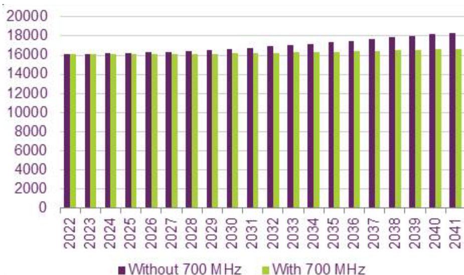
Figure 2: Analysys Mason’s estimate of the number of network sites required in the central high scenario for a generic operator
