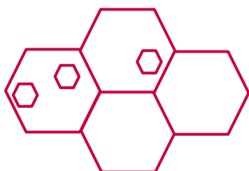
Figure 6 – Heterogeneous deployment: actual deployments will be a mix of large and small cells
