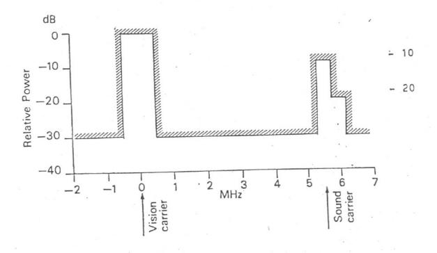
The distance from the broadcasting transmitter at which the field strength reduces to the maximum permitted by the land mobile use is thus less at frequencies between the carriers than at frequencies close to the carriers.
