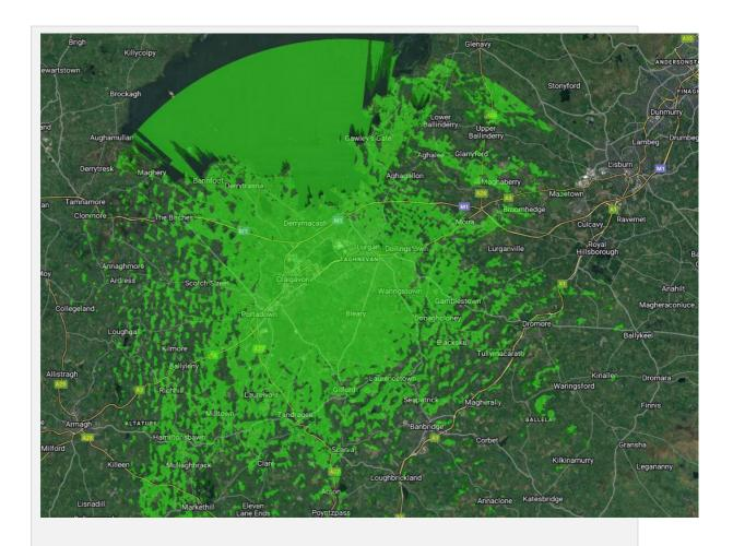
It is our assessment that the proposed transmitter site and power will provide in specification indoor coverage to a population of 76,900 persons over 15 years of age within the advertised polygon. We have compared the results from our Tower coverage mapping software to other Small scale DAB applications across the UK (including Northern Ireland) from the Ofcom website and have found the coverage population results to be within +/-5% of the various models used by other applicants.
