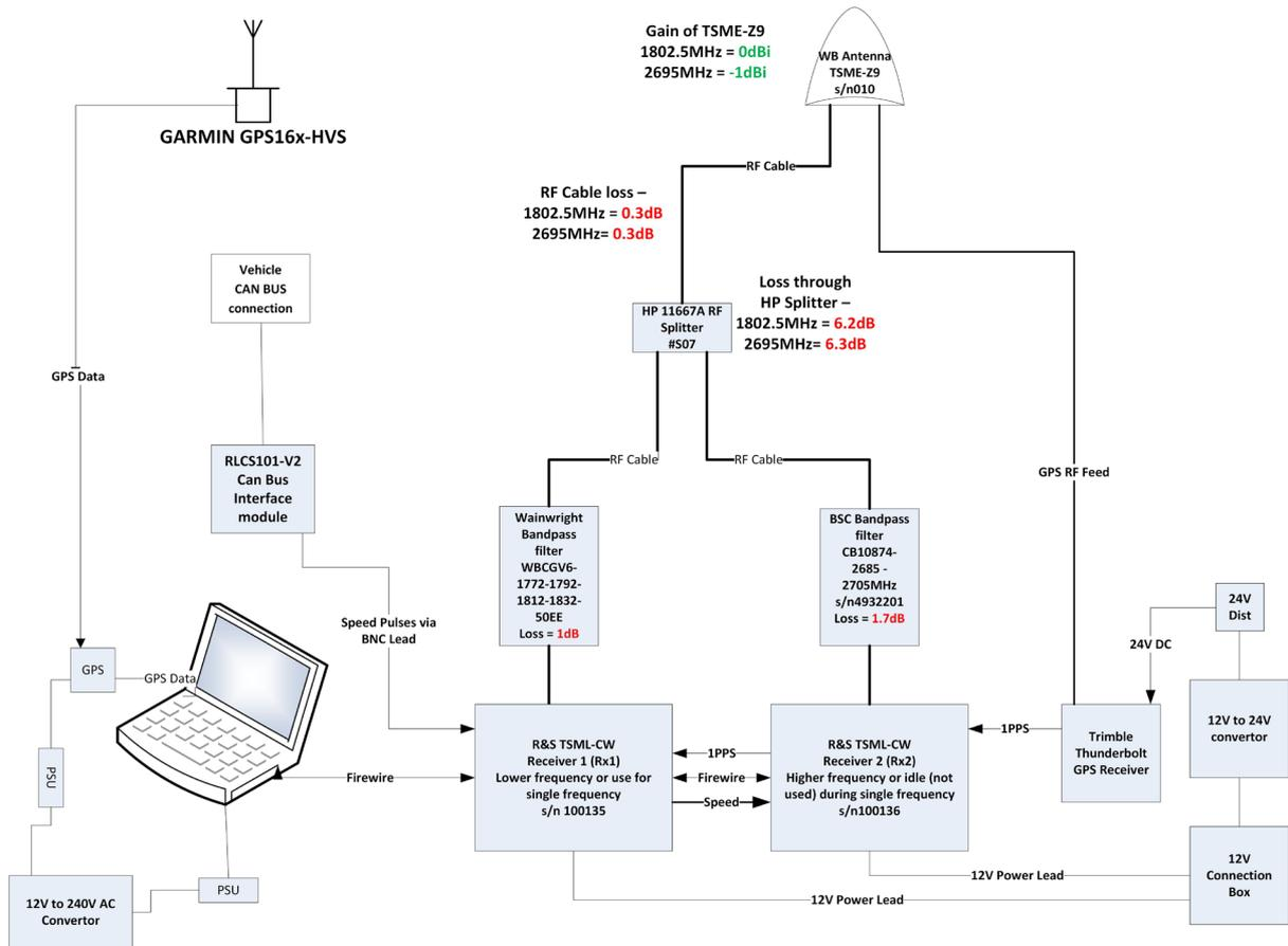
Figure A1.4: Receiver equipment configuration diagram for 5850.00 MHz in Merthyr Tydfil
