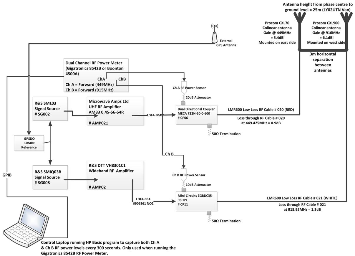
Figure A1.2: Transmitter equipment configuration diagram for 3602.50 MHz in Nottingham
